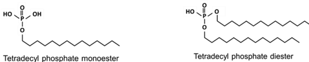
Figure 58. Molecular structures of in-house synthesized tetradecyl phosphate ester (PE-C14) (73.5% monoester & 25.5% diester) (reprinted with permission from [48]).
